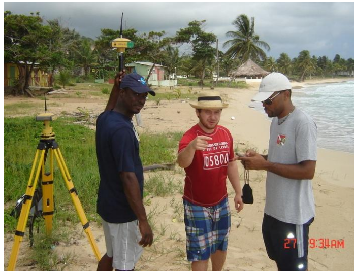
Figure 5.6.1: High Resolution Coastal Profile Surveying with GPS, Long Bay, Jamaica
