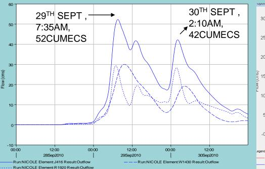
Simulated discharge at the junction node near the mouth of the river at harbour view.
