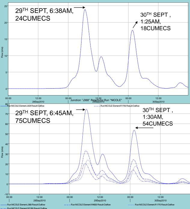
Simulated peak discharges at junction of flow nodes at the fording at Kintyre.
