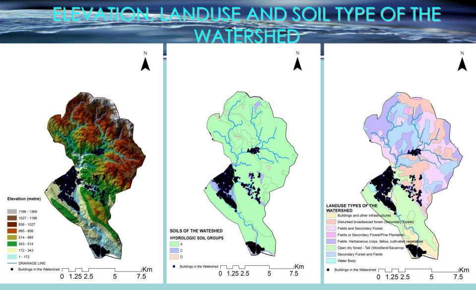
Elevation Map created from DEM of 6m horizontal and 1m vertical resolution. Note the buildings are located in the floodplains of the river and in the areas of low elevation. High elevation in the upper watersheds coupled with impermeable rocks results in less infiltration. Hence high run off and flooding in the downstream areas. Soil data shows buildings located in zones with moderate high runoff ie C.
