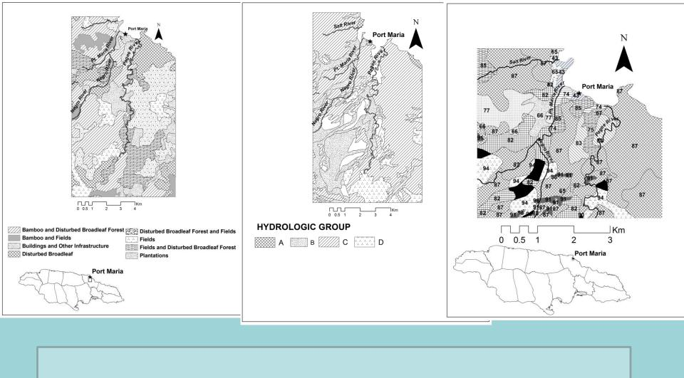
Identifying curve number for catchments using soil, landuse data in ARC GIS
