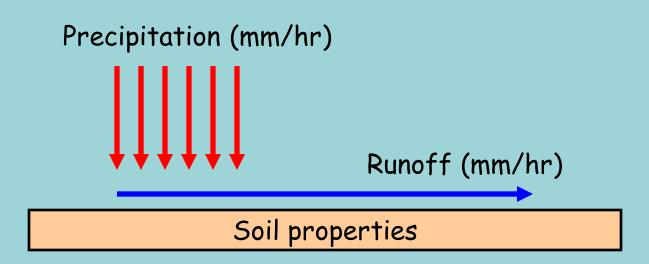
Runoff = f(precipitation, soil properties, moisture conditions)
